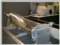
Complex Ducting Assembly Forming - Aluminum Welding Tube Bending - Assembly
